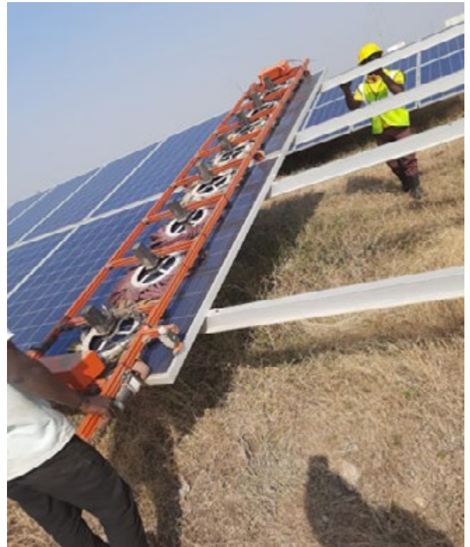
Dry robotic cleaning with microfiber cloth
